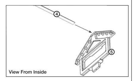
• Insert the Short Shield Knob (C) through the Sneeze Guard Side Post (5) and screw it into the Sneeze Guard Ridge Channel (4) (Do not fully tighten, leave a minimum of 1/2" exposed thread per side)
