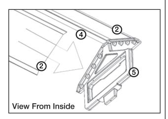
• Install and fully tighten long shield knob on each of Food Bar (B)
