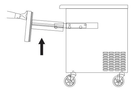
Fully extend the drawer out toward you as pictured. After full extension, lift the drawer up and pull toward you. This will disengage the rollers from the roller guide.
