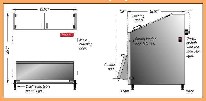
Option: .250 thick anodized aluminum loading doors.
