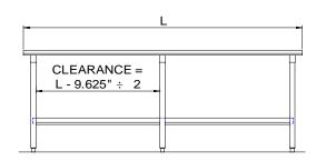
All units ship unassembled for reduced shipping cost. Units 7 ft. and larger are furnished with six legs. All dimensions are typical. Tolerance +/- .500".
