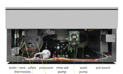
components position all service components are installed in front of the machine for easy assistance and reduce service time.
