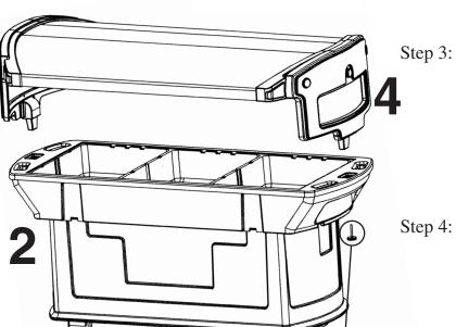
With Sneeze Guard Assembly seated securely, insert the two remaining black plastic knobs through underside of basin and screw into bottom of Sneeze Guard Posts. Tighten knobs with moderate force.
