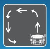
Fan placement helps to create drying pattern for hard to reach areas effected by unwanted moisture.
