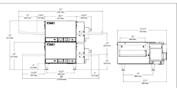
Electrical Service: Heat is supplied by one (1) element at 5600 watts. Each oven is rated at 6kW. The ovens are available in 208V and 240V and are single phase. The oven comes with a factory installed cord wth NEMA 6-50 plug. A separate circuit breaker is required for each oven deck with the proper voltage, amperage, phase and hertz as indicated by model number.
